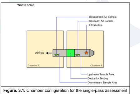
• Chamber A – downstream, contained a post-exposure duct section.
